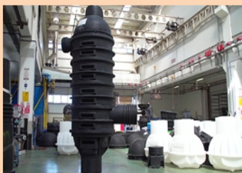
PSD Rotoworx RMPP141 manhole
